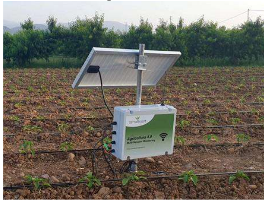
figure 66 smart plant monitoring system using iot
